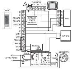
IF A THERMOSTAT OTHER THAN A TH5110, TH5220, TH5320, TH6110, TH6220, TH6320, TH8110, TH8320 OR TH8321 IS USED, A RELAY MAY BE REQUIRED TO ISOLATE THE G WIRE.
